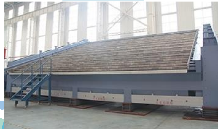
The self-developed 1,000 tonnes/day grate furnace
